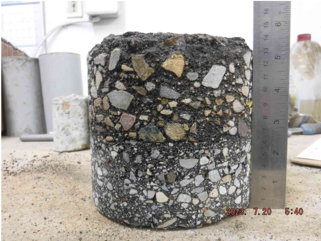
Photograph 1: Asphalt core from the location of BH23-2
